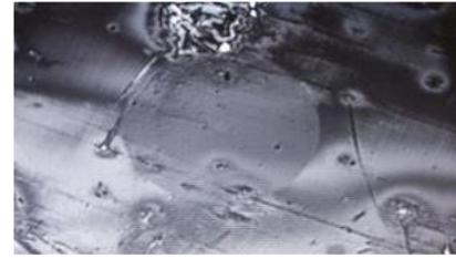
Figure 6 - Dry cleaning tends to move debris
